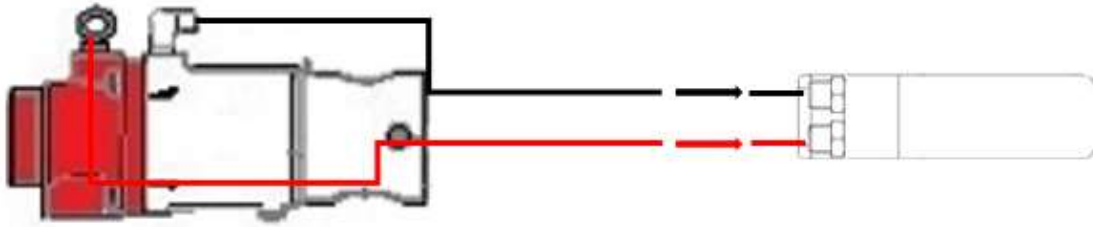
Figure 5.3 – Remote Control Valve with Pneumatic Deadman Controls
